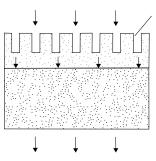
Surface structure spreads water flow and increases filtration area.
